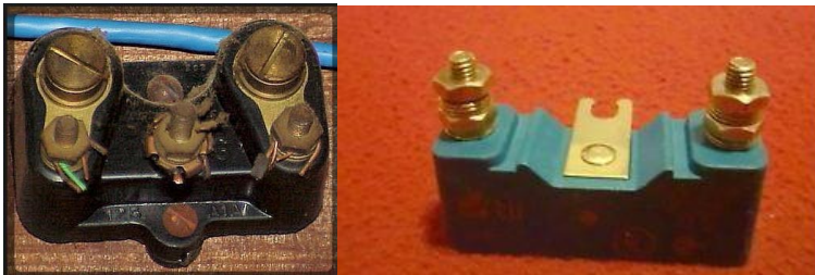
Small devices: Big impact. Left: Typical carbon protector by Western Electric ($1). Right: Gas tube protector by TII ($3)
